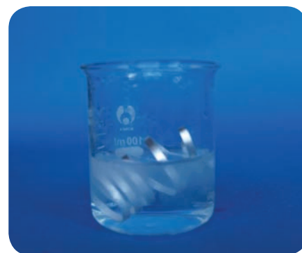
▲ Magnesium displacing hydrogen from hydrochloric acid.
