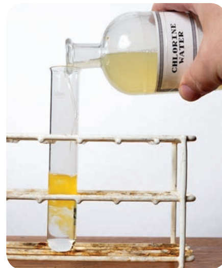
▲ Chlorine displacing bromine from aqueous potassium bromide.
