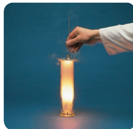
▲ Sodium burning in chlorine, to form sodium chloride.
