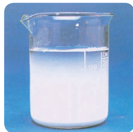
▲ A mixture of chalk powder and water. This is not a solution. The tiny chalk particles do not separate and spread through the water particles. They stay in clusters big enough to see. In time, most sink to the bottom.
