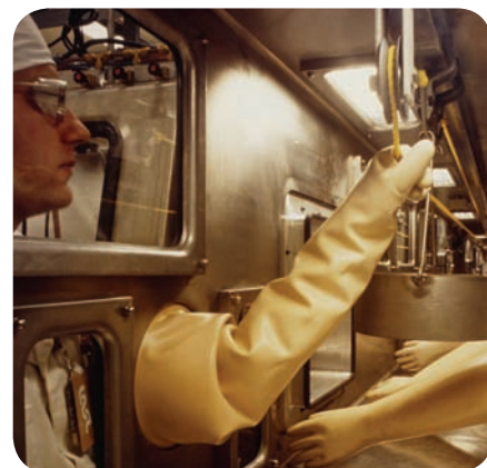
▲ Radioisotopes are dangerous. This scientist is using a glove box, for safety.
