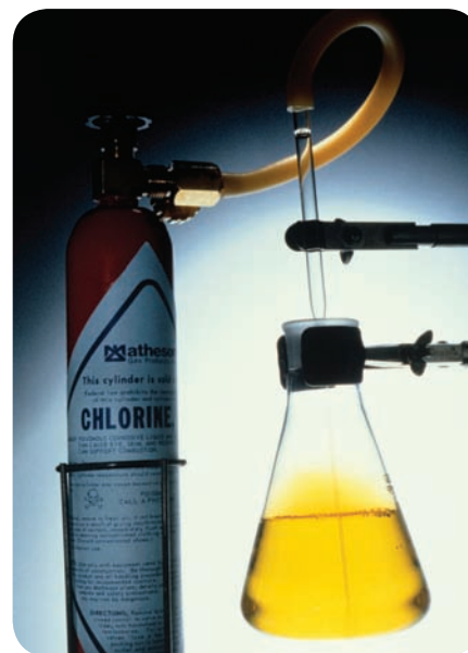
▲ Bromine being displaced by chlorine, from a colourless solution of potassium bromide. The solution goes orange.
